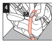
Push down firmly on the child restraint and pull up on belt to tighten. For a manual belt, refer to "Knowing your Vehicle Belt" section. Pull up on shoulder strap to remove any slack.
